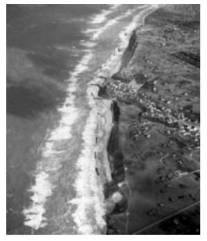
*Fig. 7: Nourishment, revetment and breakwaters.*
